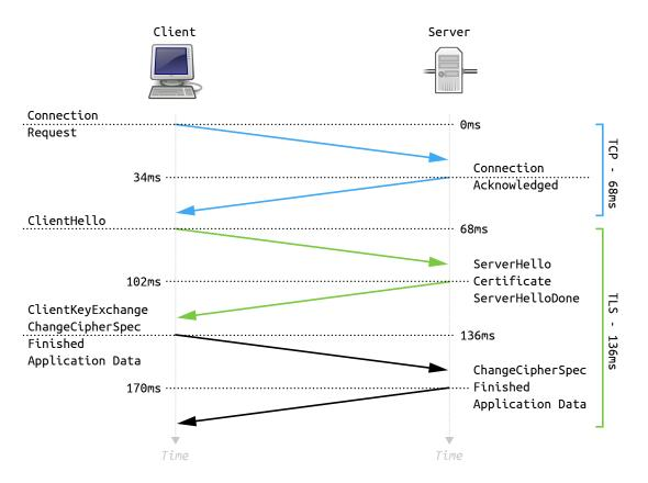
Figure 15: TLS False Start handshake (Fussenegger 2015h).
