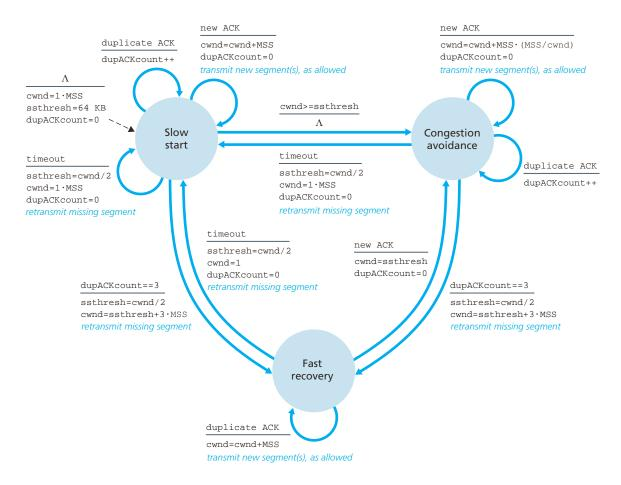
Figure 4: Finite state machine illustrating TCP's slow-start, congestion avoidance, and fast recovery coherences (recreated from Kurose and Ross 2013, 275)
