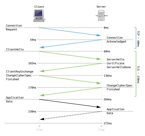
Figure 10: Full TLS 1.2 handshake (Fussenegger 2015c).
