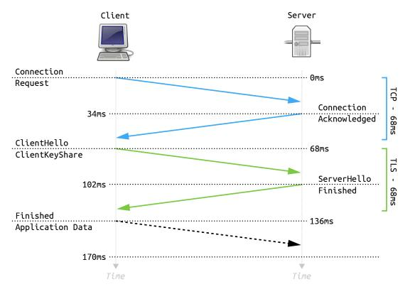
Figure 14: Abbreviated TLS 1.3 handshake (Fussenegger 2015g; Rescorda 2015b, 33).
