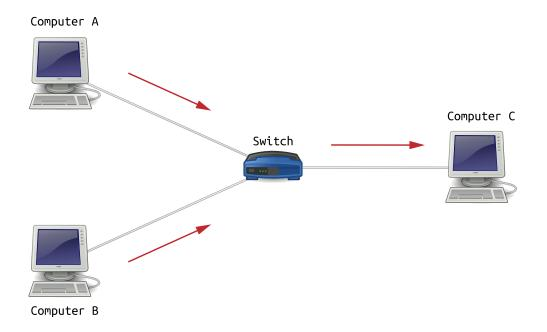
Figure 1: Switch with three computers attached, and arrows that indicate in which direction the streams move (Fussenegger 2014e; Kurose and Ross 2013, 36, Figure 1.16).
