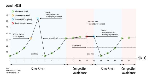
Figure 3: Illustration of TCP's slow-start and congestion avoidance (Fussenegger 2014b; Inacon GmbH 2010).
