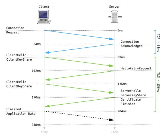
Figure 13: Full TLS 1.3 handshake with mismatched parameters (Fussenegger 2015f; Rescorda 2015b, 32).
