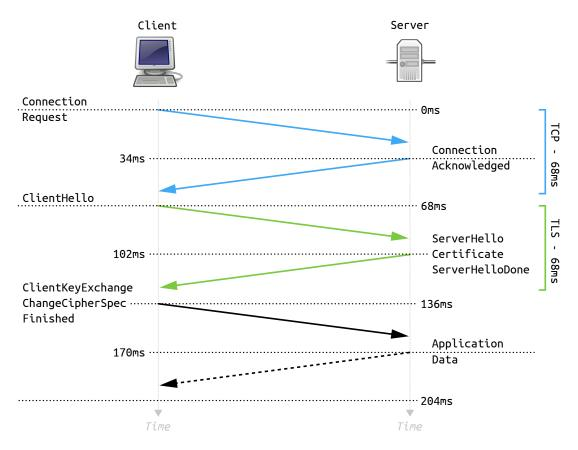
Figure 11: Abbreviated TLS 1.2 handshake (Fussenegger 2015d).
