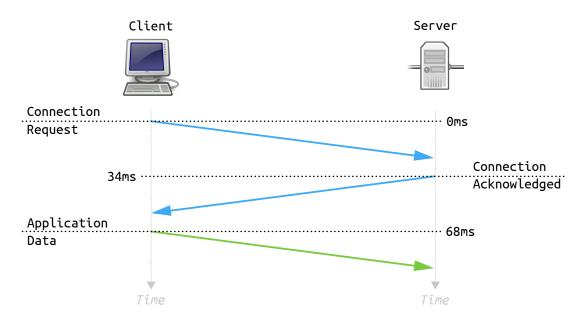
Figure 2: Simplified illustration of the TCP 3WHS with timing information from the example calculation in section 2.1.1 (Fussenegger 2014a).
